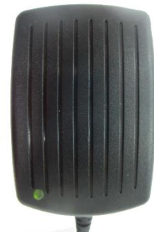
Battery Charger Fully Charged
