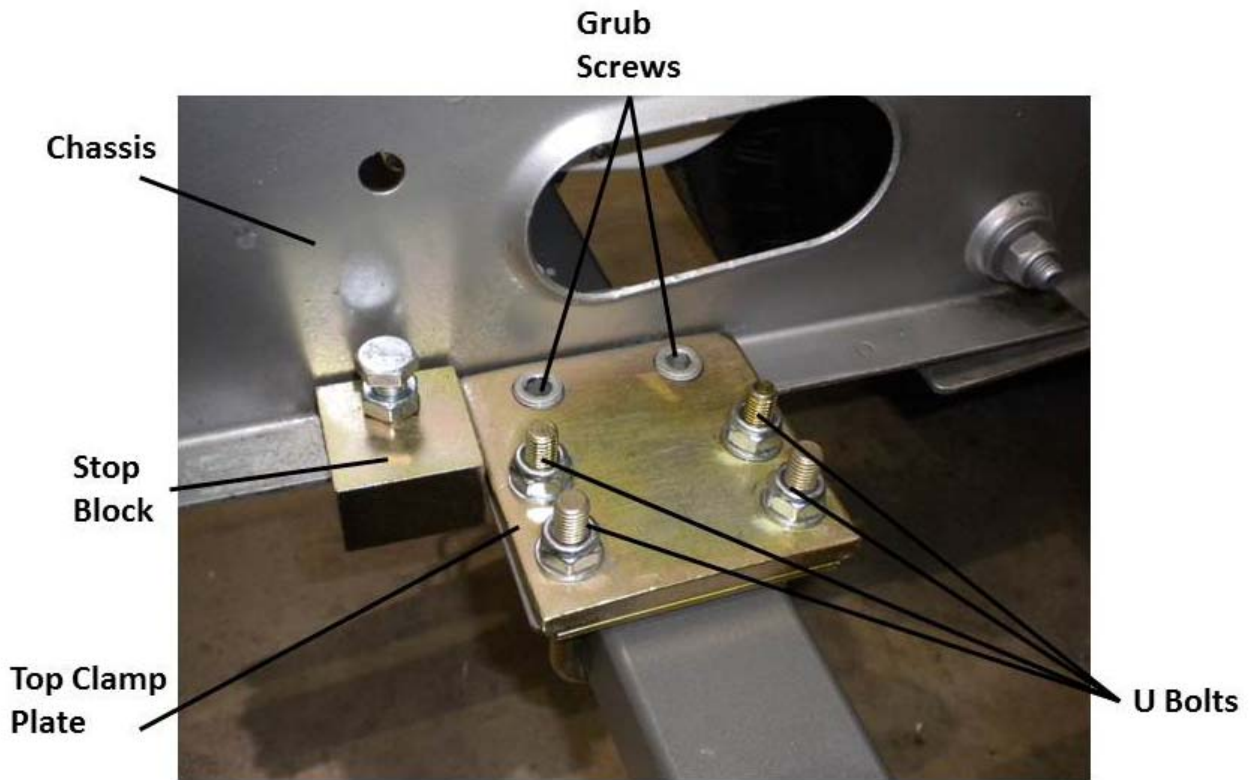
FIG 3: CLAMP ASSEMBLY WITH STOP BLOCK
