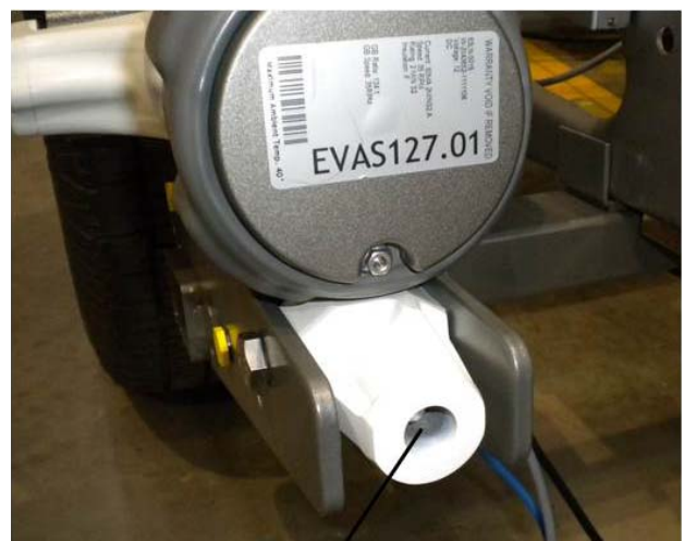
Evolution end view Showing position for T bar after end bung has been removed
