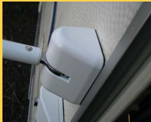
Fit 2 x Gaskets and then tighten 8 x M6 screws.
