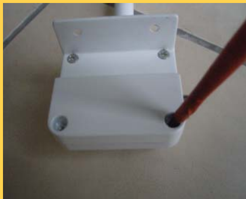
Check orientation and screw frame mounting kit to Security Handrail.
