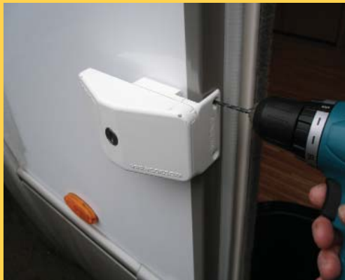
Drill 2 holes 4.5 Diameter
