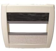
Aperture Roof thickness Corner radius Site dome Height over roof Ventilation Weight Size inner frame Outer frame material Dome material Speed limit Authorization 400 x 400 mm 24-56 bzw. 42-70 mm 23 mm 560 x 560 mm 92 mm 150 / 30 cm² 3,0 kg 565 x 530 x 35 mm Polypropylene Polypropylene 130 km/h ECE R43 -019649
