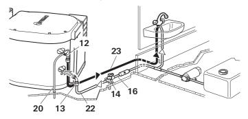
Slide elbow fitting (13) onto cold water connecting pipe (lower pipe) and elbow fitting with integrated ventilating valve (12) onto hot water connecting pipe (upper pipe) of water heater as far as it will go. Pull in opposite direction in order to make sure the elbow fittings are securely attached.
