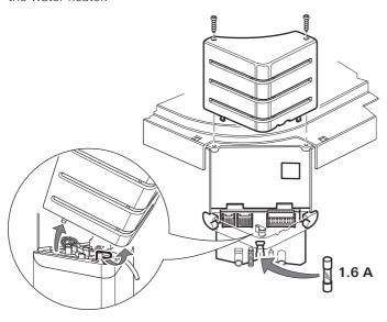
Only replace the miniature Fuse on the p.c.b. with a fuse of the same type: 1.6 A, EN 60127-2-3 (slow action).
