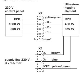
Correct connection of L and N line to the corresponding power supply lines must be ensured for safe operation.
