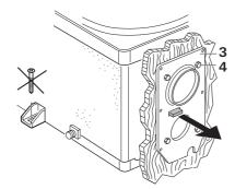
Screw the sealing frame (3) in contact together with the cowl body (1) so the anti-twist device projects out!
