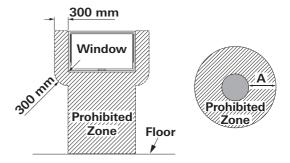
The heater must not be installed close to or directly behind a room / space heater.
