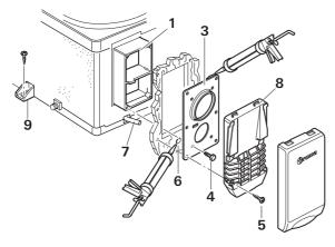
Seal the gap between the hole (6) and the condensation tube (7) with non hardening mastic – do not use silicone!
