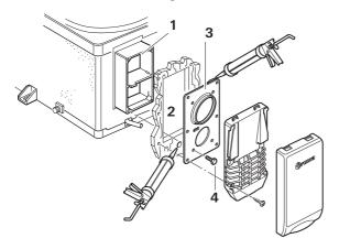
Remove sealing frame (3) and coat with non hardening mastic on the side facing the vehicle – do not use silicone!
